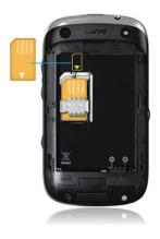
Slide the SIM card into the slot.
